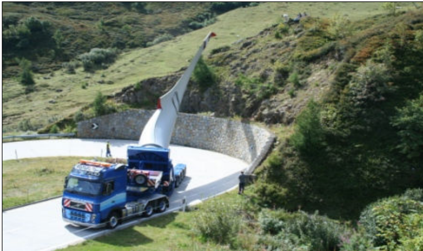
Plate 4-5 Blade adaptor transport system
